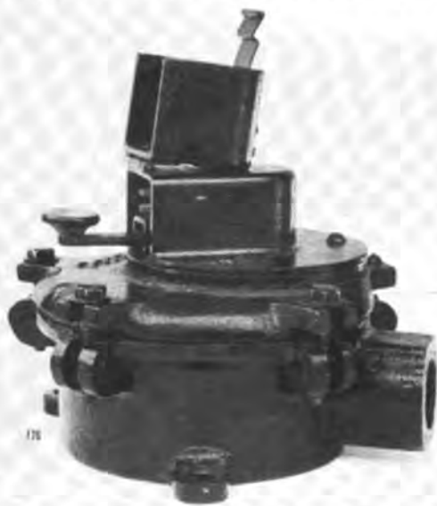
● (176) Key used by U.S. Military in WW-II. No markings. Nicknamed "The Pressure-cooker" by Elwood's XYL/Edith. Small key mounted in flame-proof compartment. Heavy construction.
